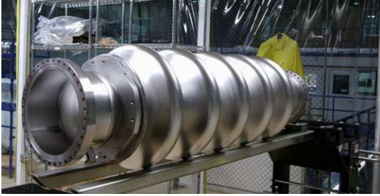
Figure 5: The ERL cavity following BCP at JLab.
