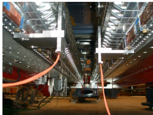
Figure 1: Radiator of the APPLE II type in operating position without vacuum chamber. Four power meter sensors (see below) at each undulator end (orange cable) are installed.
