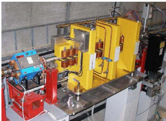
Figure 3: The radiator which causes horizontal oscillations.
