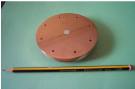
Figure 5: Mg film deposited over the backflange of a BNL/SLAC/UCLA 1.6 cells S-Band RF gun.
