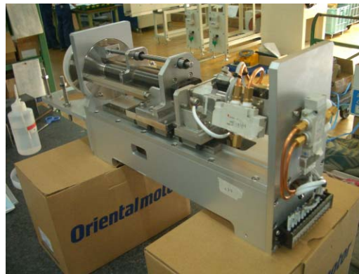
Figure 7: The drive assembly of the Cherenkov radiator with a two-staged stroke. The first stage is a profile monitor with a fluorescence ceramic screen, and the second stage is the Cherenkov radiator with the aerogel.
