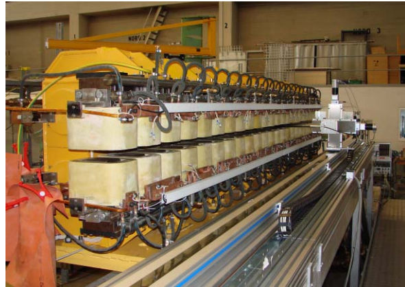
Figure 1: View of the infrared undulator on the DESY magnetic field measurement bench
