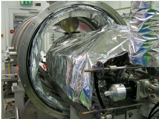
Fig. 7: Photograph of the vacuum vessel and the He vessel during moving in.
