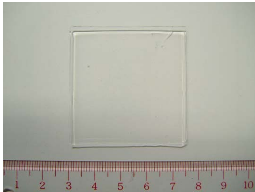
Figure 5: A thin hydrophobic silica aerogel used as a Cherenkov radiator with a thickness of 1.5 mm and the refractive index of 1.05.
