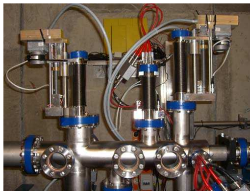
Figure 5: Layout of MCP detector with extended wavelength range installed at FLASH in 2007 (MCP07). Detection of backward reflected radiation is performed with stationary mounted MCP1 and MCP2. MCP3 and MCP4 are movable. When positioned off-axis they measure small angle reflected radiation. Measurements of direct photon beam is also possible when positioning MCPs on axis. MCP5 detects radiation reflected by Fe mirror. Target unit contains four grids of different materials (Au, Cu, Fe), and light attenuator.
