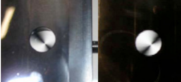
Figure 3: Radial polarization converter (ARCoptix, Switzerland) based on liquid crystal: Comparing the right and left (rotated 90 degrees from each other), it is clear that the converter generates a radial polarization.
