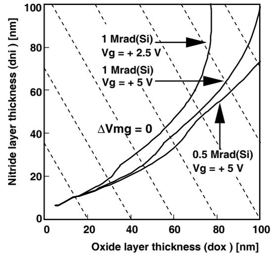
Figure 6: The optimum insulator thicknesses of MNOS structures with different radiation conditions when  $V_g > 0$ . The equivalent oxide thickness is the same on each dashed line.
