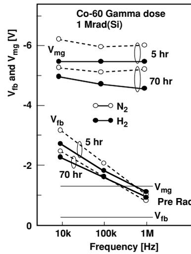
Fig. 2:  $V_{mg}$  and  $V_{fb}$  of MOS structure before and after irradiation.
