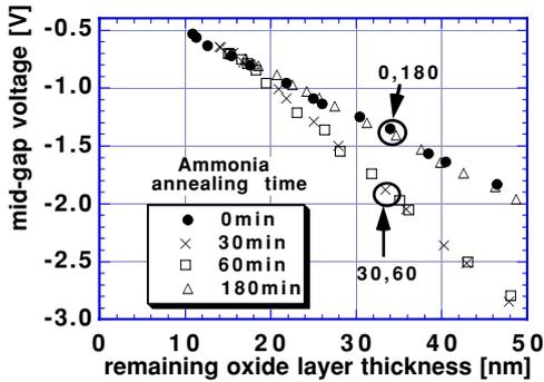
Fig. 12: Midgap voltages distribution of MOS structure after irradiation.
