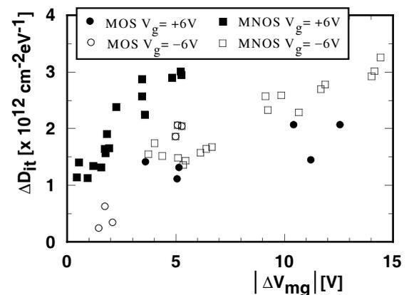
Figure 3: Radiation-induced  $D_{it}$  shift in MOS and MNOS structures as a function of the magnitude of  $V_{mg}$  shift.
