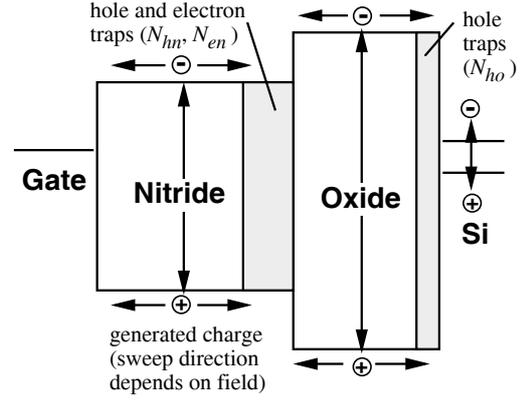
Figure 4: Charge generation and trapping model of MNOS structure under irradiation.
