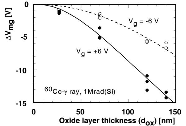
Figure 1: Radiation-induced  $V_{mg}$  shift of MOS structures. Points show the experimental results. Lines show the calculated results.
