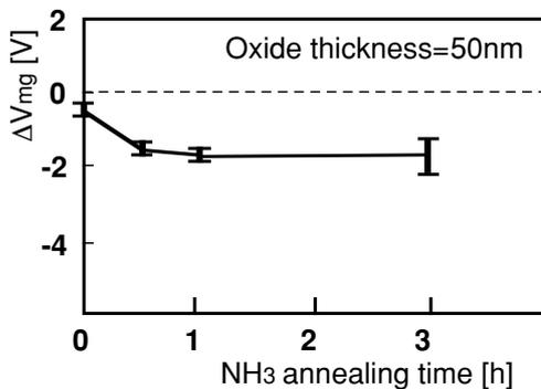
Fig. 7: ΔV<sub>mg</sub> of ammonia annealed MOS capacitors after irradiation.
