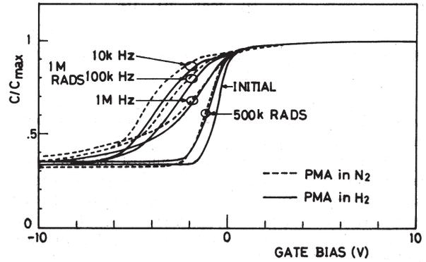
Fig. 1: C-V characteristics of MOS structure before and 5 hours after irradiation.
