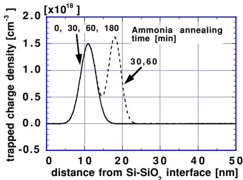
Fig. 13: Estimated charge profile in oxide layer annealed in NH<sub>3</sub> after irradiation.
