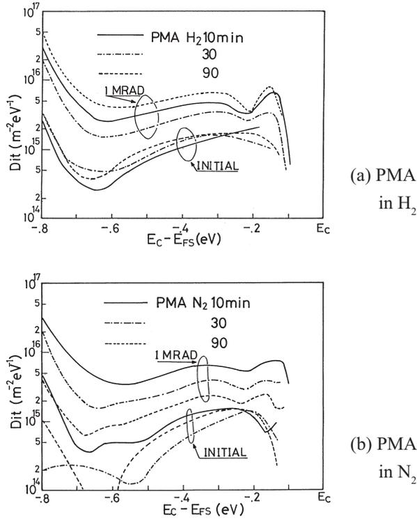
Fig. 3: Si-SiO<sub>2</sub> interface states densities (Dit) of MOS capacitors PMA in H<sub>2</sub> (a) and in N<sub>2</sub> (b).
