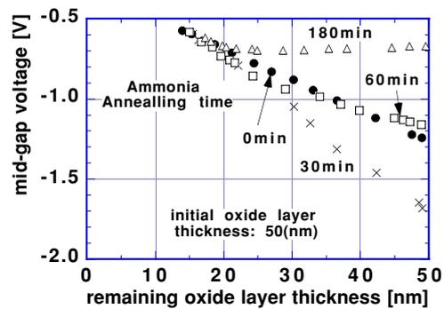
Fig. 10: Midgap voltages of the MOS capacitors prepared by slanted etching method.
