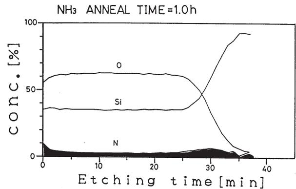
Fig. 9: Composition of the oxide annealed in NH<sub>3</sub> at 950 °C analyzed by XPS.
