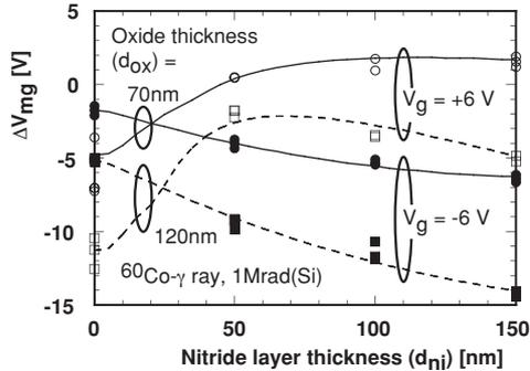
Fig. 16:  $\Delta V_{mg}$  of MNOS structures due to irradiation.
