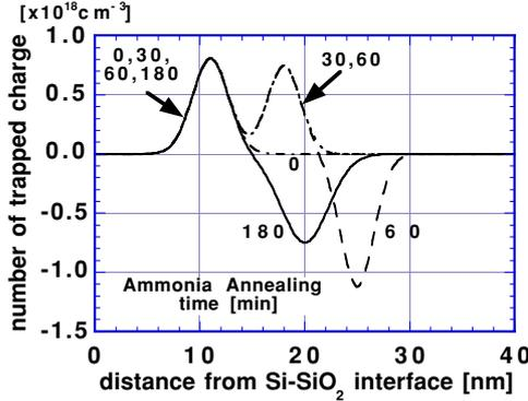
Fig. 11: Estimated charge profile in oxide layer annealed in NH<sub>3</sub> before irradiation.
