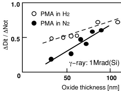
Fig. 5: ΔDit/ΔNot for the cases PMA in N<sub>2</sub> and in H<sub>2</sub>.
