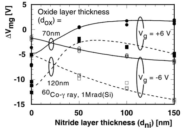
Figure 2: Radiation-induced  $V_{mg}$  shift of MNOS structures in which the oxide thicknesses are 70 and 120 nm. Points show the experimental results. Lines show the calculated results.
