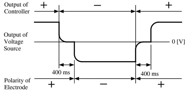
Fig. 3. Time chart of alternately changed polarity of voltage (AC).
