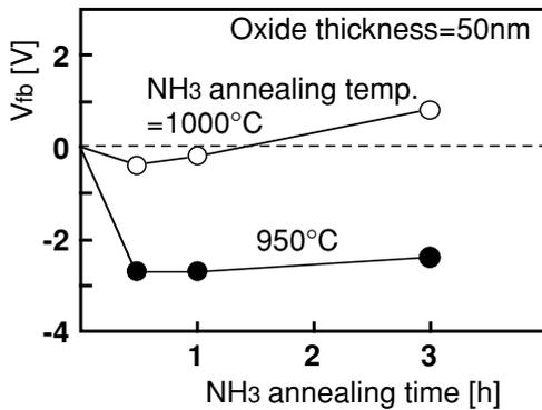
Fig. 6: V<sub>fb</sub> characteristics of MOS capacitors annealed in ammonia at 950°C and 1000°C.
