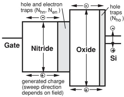
Fig. 14: Charge generation and trapping model of MNOS structure by ionized irradiation.
