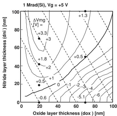
Fig. 17: Simulated  $\Delta V_{mg}$  of the MNOS structure.
