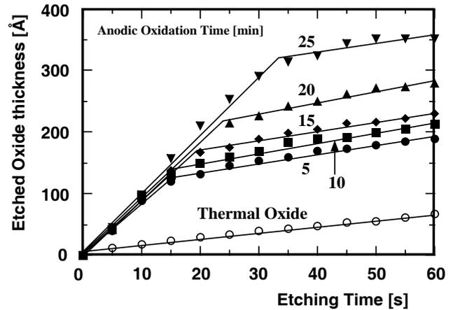
Fig. 6. Etched oxide thickness vs etching time for different anodic oxidation times.
