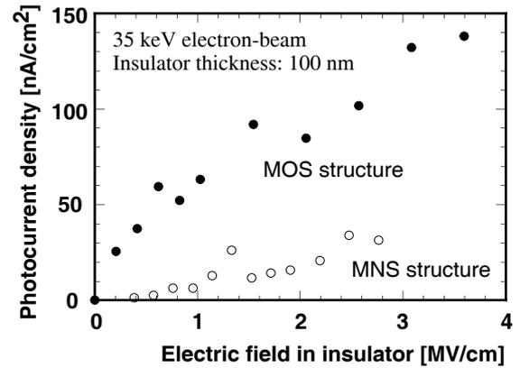
Figure 5: 35 keV electron-beam photocurrent densities of MOS and MNS structures as a function of electric field.
