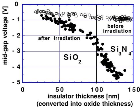
Fig. 15:  $V_{mg}$  of MNOS capacitors before and after irradiation.
