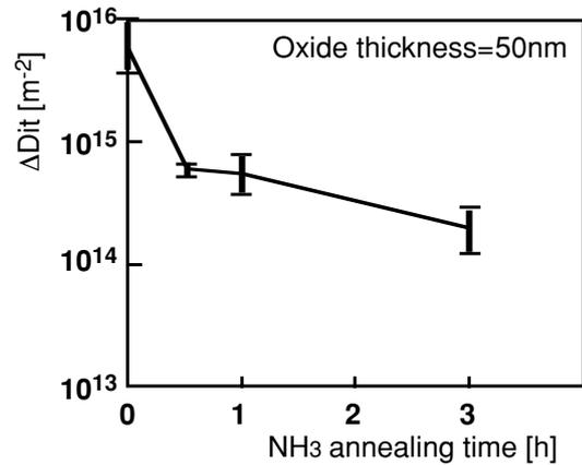
Fig. 8: ΔDit of ammonia annealed MOS capacitors after irradiation.
